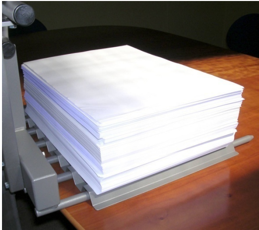
Figure 13 – Position of forks before lifting pallet and paper.
