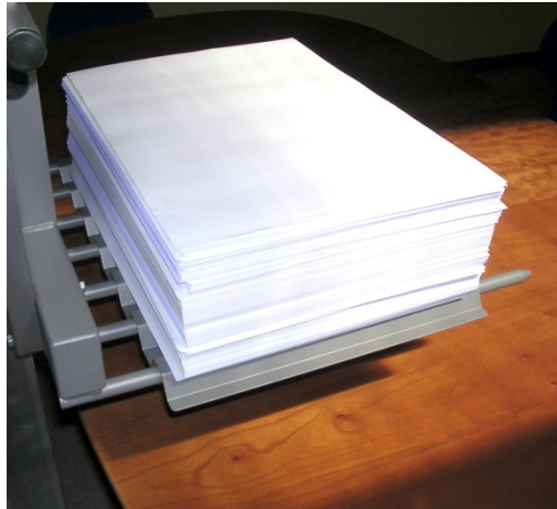
Figure 14 – Lifting paper on pallet.
