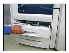
2. Load the envelopes in the envelope tray with the flaps closed, flaps down, and on the leading edge (toward the left).
