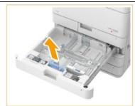
Attach the Envelope Feeder Attachment A by aligning the protruding areas with the holes located on the bottom of the paper drawer.
