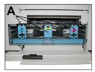
5. Insert Ink Tanks (labels up) into appropriate color slots [B]. Close three Ink Tank Latches. INSTALLATION TIP: Make sure Ink Tanks seat properly. Insert Ink Tank into appropriate Ink Station, then pull Ink Tank back about an inch and push forward firmly to insure that Ink Nozzles penetrate seals on Ink Tanks.
