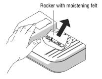
· Slightly tilt the rocker and pull it off in an obliquely upward direction.
