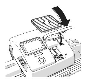
Close the flap of the print system by pushing it down on the lower right corner.
