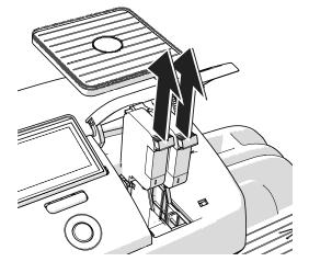
Take both ink cartridges upward and out of the socket.
