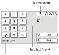
Button assigned acc. to function (here: reset to current date)
