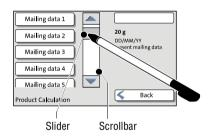
You can operate scrollbars with the arrow buttons or by touching the slider and moving it. The setting is updated when you lift your finger off.
