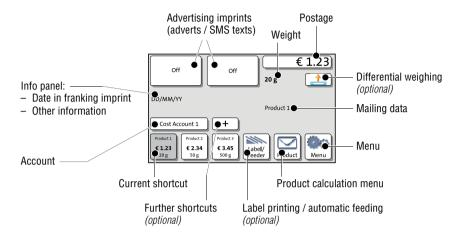
The Home screen appears after the machine was turned on and the start routine has been successfully completed. It displays the current franking settings. The postage appears only when all required product details are selected and the set weight exceeds 0 g (0 oz).
