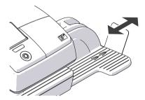
• The catch tray can be adapted to different envelope sizes by displacing the catch bracket. The stop features several catches for the most common sizes.
