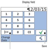
Button assigned according to function (here: reset to current date)
