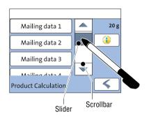
You can operate scrollbars with the arrows or by touching the slider and moving it. The setting is updated when you lift your finger off.
