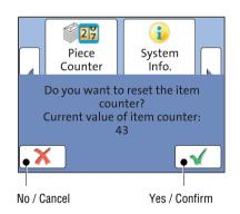
For some settings, a window covering parts of the current window opens (pop-up window). The pop-up prompts you for an action. Messages and the 'PC Mode' (using the PC control software for PostBase Mini) also appear as a pop-up.
