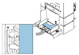
Turn the envelope support to distribute the weight of the envelopes evenly on both 8. sides.
