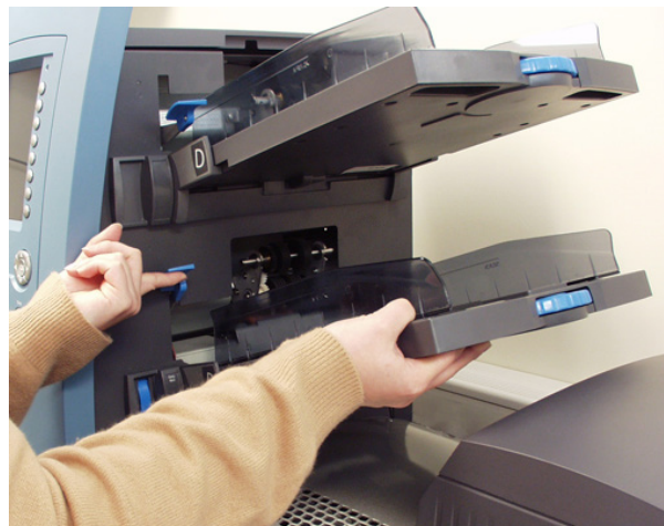
Lift the separator and slide tray into tray mounts
