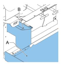
2. Remove the sealing liquid reservoir **B** from the system.
