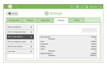
The BCR 1D code definition screen shows only information when a configuration sheet is read. It shows which codes are enabled and how they work.
