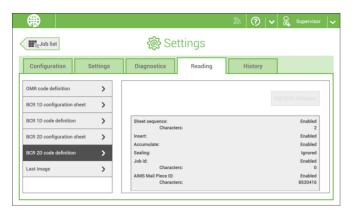
The BCR 2D code definition screen shows only information when a configuration sheet is read. It shows which codes are enabled and how they work.
