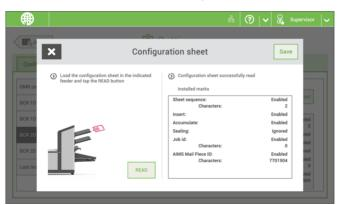
The Reading BCR 2D configuration sheet allows you to read a configuration sheet. The result is visible in this screen, but also in the BCR 2D code definition screen. See Reading a configuration sheet on page 104.
