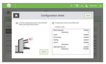
The Reading BCR 1D configuration sheet allows you to read a configuration sheet. The result is visible in this screen, but also in the BCR 1D code definition screen. See Reading a configuration sheet on page 104.
