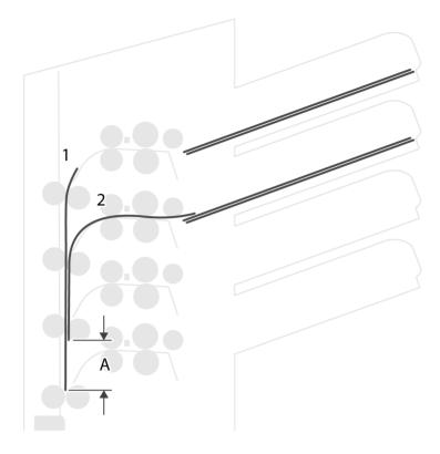
• BRE offset: in the case of offset is "yes", the last document that was added to the set is shifted from the rest of the set (offsetting, see below).
