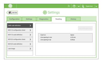
The Reading OMR code definition screen shows the configuration of the system for OMR. For every OMR code option, it shows if it is on or off. If it is on, the screen shows information on what the system does, when it reads a mark or no mark.
