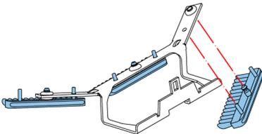
4. Replace the brushes. Make sure that the studs on the brushes are fitted in the corresponding holes in the brush holder.
