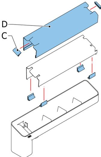
4. Remove clips **C** to remove the moistening cloth.
