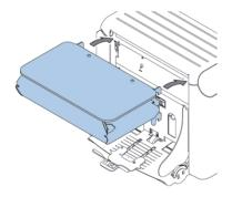
The system can be equipped with a side exit and catch tray. The side exit can be fitted instead of the envelope receiving tray. The side exit allows a conveyor or a franking system to be fitted in line with the system.
