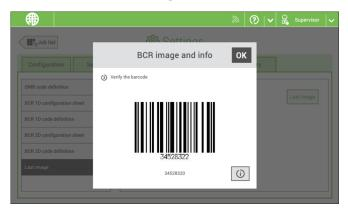
The Last image screen shows the result of the last code that the system read. The figure shows an example of the image of an OMR code. You can use this image to see if the read code fits within the reading window.
