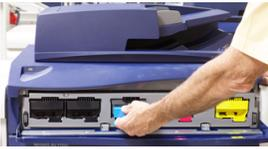
4. Remove the dry ink/toner cartridge by slowly and gently pulling it straight out. While pulling out, hold the bottom of the cartridge with your other hand to give it support.
