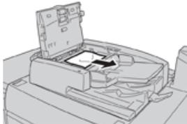
4. If instructed to open the inner cover, lift up the lever, and open the inner cover. Remove the jammed document.
