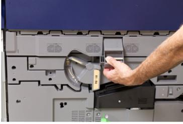
7. Remove the old drum cartridge by holding the finger rings provided at the both ends of the drum cartridge and gently lifting up.
