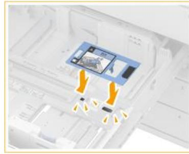
Load the envelopes with the front side of the envelopes (the side without the glued areas) face up. Load up to 50 envelopes at a time.
