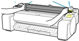
Insert the edge of the roll in the feed slot and advance the paper until the feed tone can be heard.
