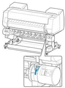
3. Hold flanges (A) so roll holder's white gear is on left, align roll holder shaft with roll holder slot left and right guide grooves (B), load.
