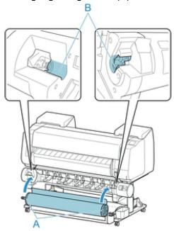
4. Change Roll Holder Lock switch to locked position.
