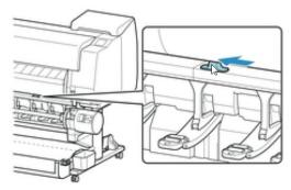
6. Begin rolling the paper down with leading edge between roll paper and arrows (A) directly beneath it, and feed roll paper until a sound is heard.
