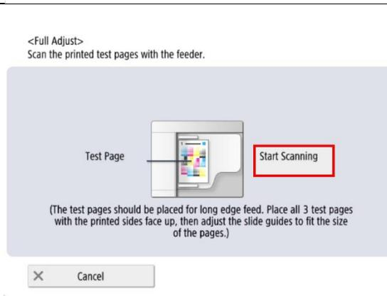
11. The adjustment may take a few minutes, when completed the machine says **<Full Adjust> Adjustment is complete**.
