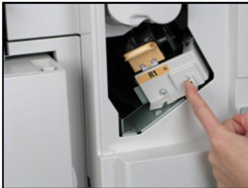
5. Grasp the Staple Cartridge by the orange handle and remove the cartridge by pulling it toward you.
