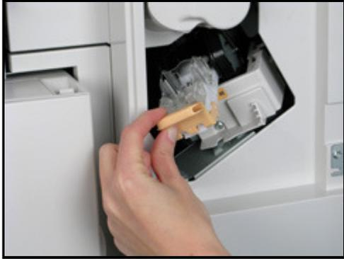
6. Remove any loose staples or other debris from inside the Finisher.
