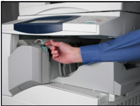
2. Remove the Staple Cartridge by grasping the cartridge by the orange handle and pulling it straight out of the Finisher.
