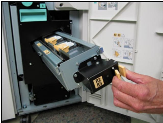
4. Grasp the orange tabs on both sides of the Staple Cartridge, rotate slightly to the right, and lift the cartridge out of the Staple Cartridge Unit.
