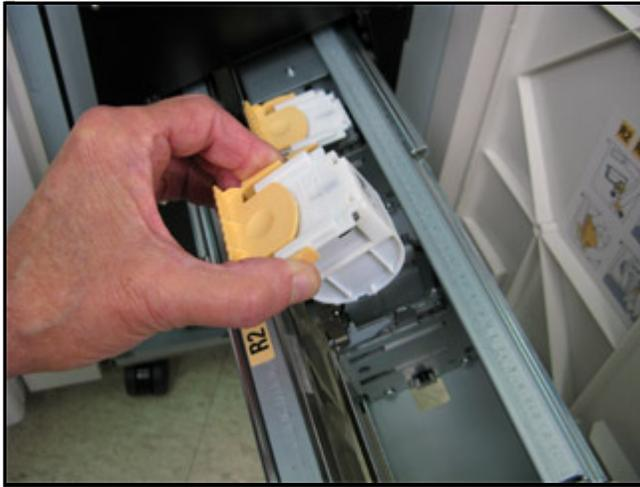
5. Push the new cartridge into the Staple Cartridge Unit.
