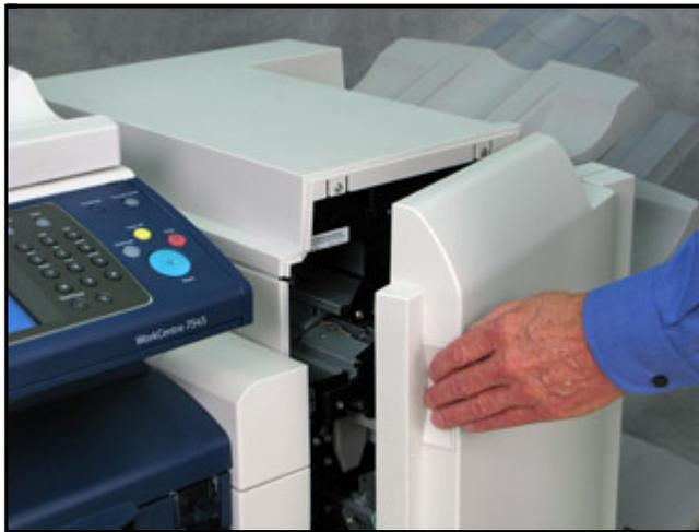
3. Squeeze the orange R2 and R3 levers together and pull the Staple Cartridge unit out of the Finisher until it stops.
